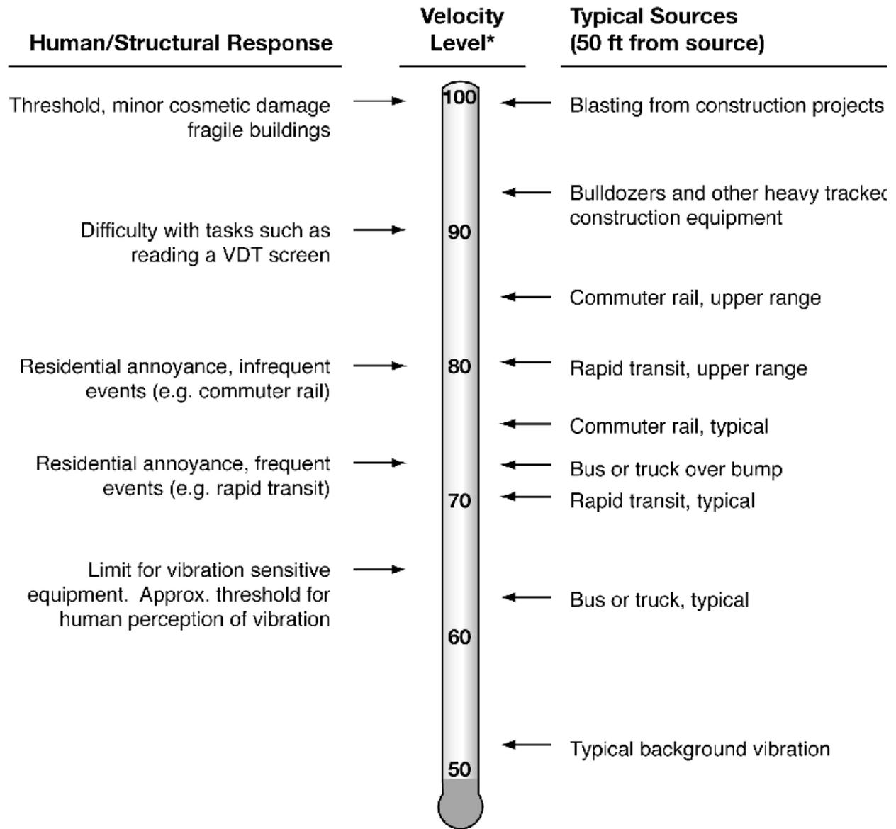
\* RMS Vibration Velocity Level in VdB relative to 10<sup>-6</sup> inches/second
